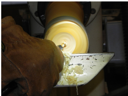
After removing the tailstock, the tool rest is drawn close to the end of the goblet.
