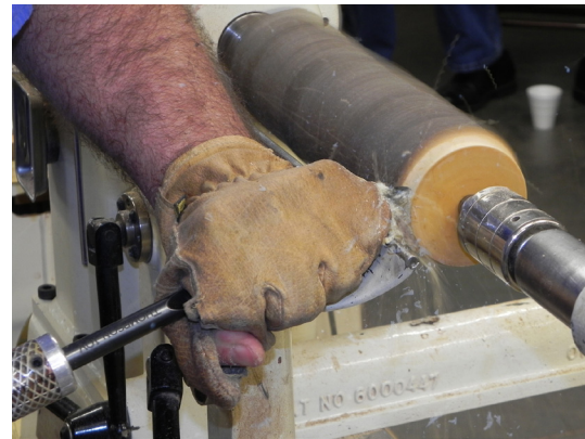
Using a spindle gouge, he create a tenon to mount the limb on a chuck.
