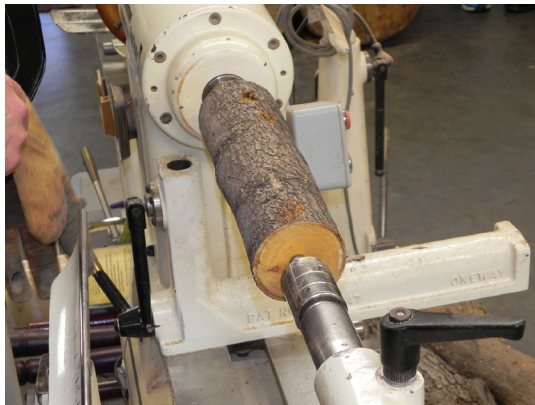
Randy started mounting the limb between centers.
