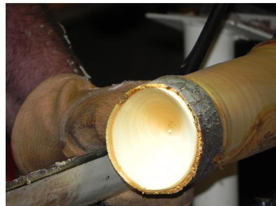
Turning end grain, Randy used a spindle gouge to hollow inside the cup.
