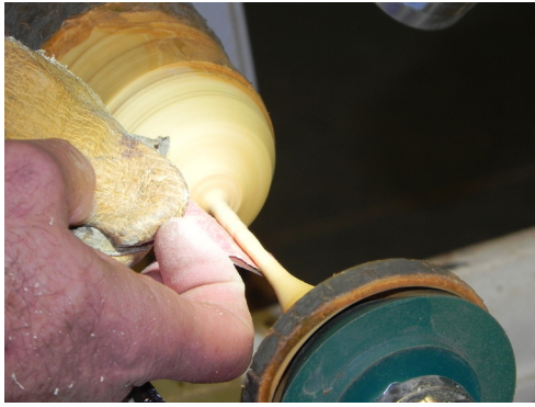
Sanding the fragile stem lightly.
