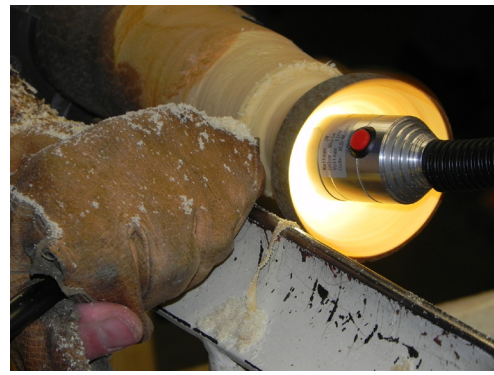
To turn the cup as thin as comfortable, Randy used a LED light inside.
