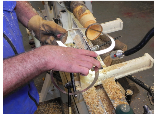
If a light is not handy, old school calipers work just as well.
