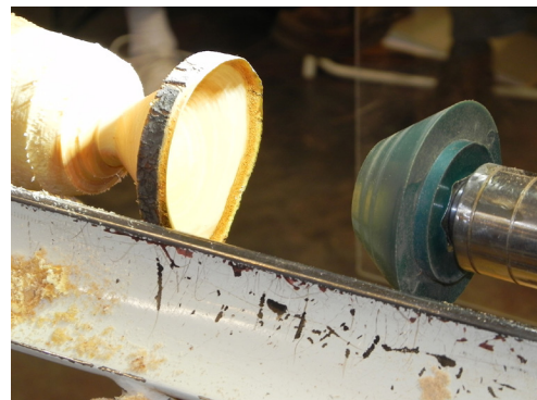
To help support the cup while turning the stem, Randy used a "Rubber Chucky". ( www.rubberchucky.com )
