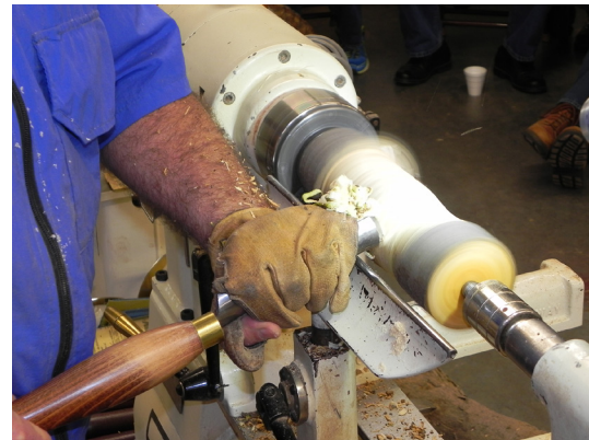
...he roughed the limb round and removed bark using a spindle roughing gouge.
