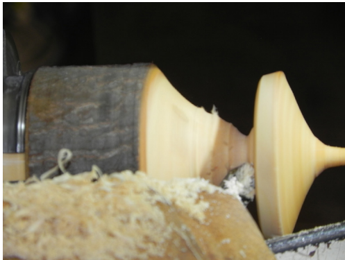
Randy only needs to undercut the base slightly to make sure it sits flat and part off the completed goblet. Almost there...
