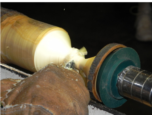
Using a spindle gouge, and very little pressure, he defined the stem.
