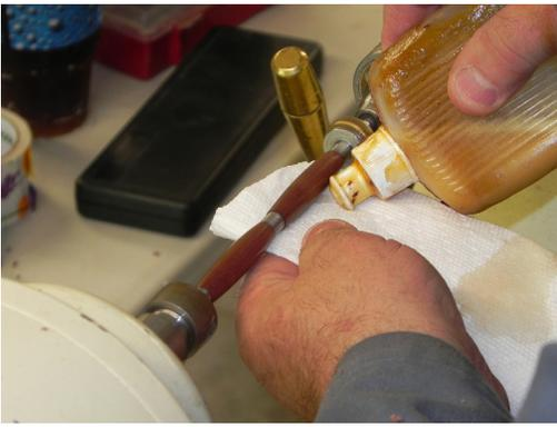
For wood pens, while the lathe is running - Apply a coat of sanding sealer by applying some sealer to white paper towel and moving it along the blank - allow it dry.
