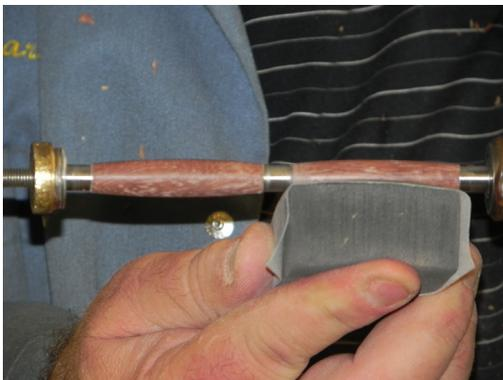
Once you have the desired shape of your pen, start the finishing process by sanding – start with 150 grit – Move the sanding strips rapidly back and fourth so you don't leave sanding rings.
