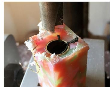
Glue in the pen tubes – use accelerator to speed up the process and mill the ends of the blanks with the pen mill.
