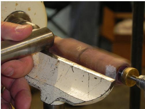
Gently start rounding out the blank – start with the edges of each blank.
