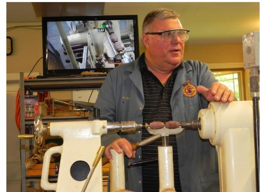
Your only constraint is that the wood diameter at the ends of the blanks needs to match the bushings. You can do whatever you want between the bushings
