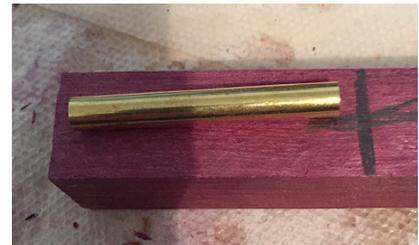
Use the tube to determine the length of each blank – add 1/8 to 1/4 inch to each end.
