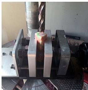
Drill the proper hole in the center of each blank.
