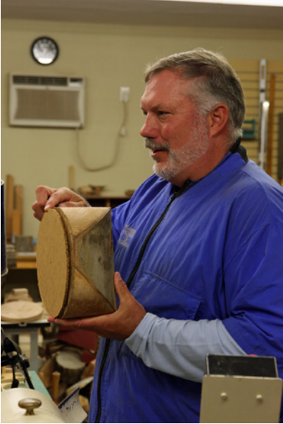
A cardboard template is used to help cut the bowl blank
