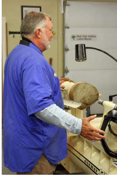
Blank is mounted on a screw center chuck
