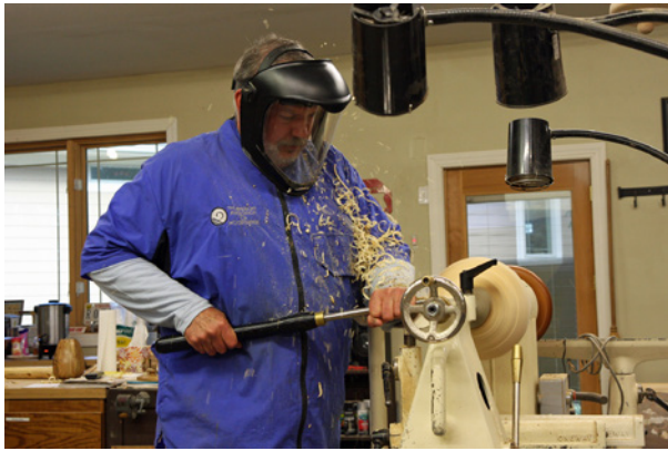
With a bowl gouge, shape the outside.
