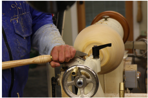
Turning a tenon to mount bowl in a 4 jaw chuck.
