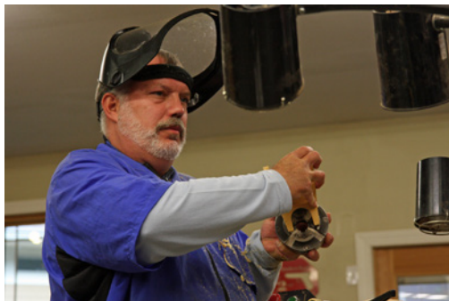
To make sure the tenon is the right size for the chuck, Randy uses a shop made gauge.
