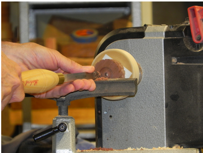
David uses double stick tape to secure wheel before turning a hub.
