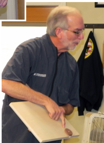
David's jig and sanding platform used to make wheels perfectly round.
