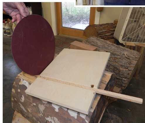
David's jig and sanding platform used to make wheels perfectly round.
