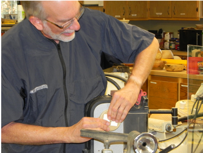
David uses double stick tape to secure wheel before turning a hub.
