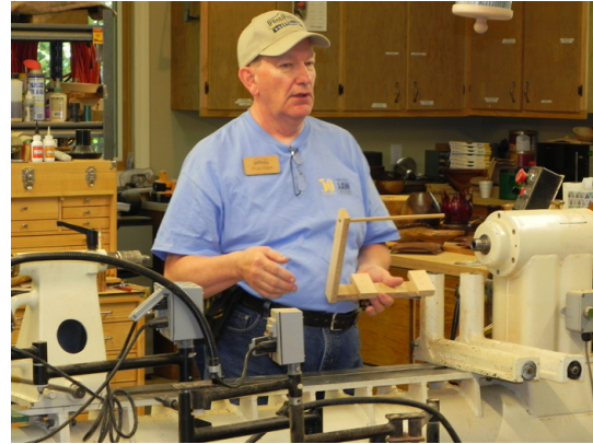
Ross Hirst shared his shop-made depth gauge to measure the depth of bowls while still on the lathe.
