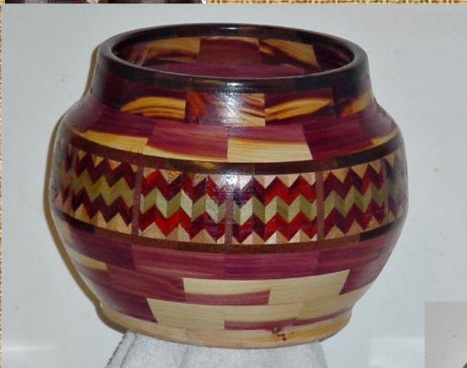
This small Pot has a feature ring consisting of padauk, poplar, maple and ipe. Body is cedar with walnut ring on top. The feature ring is made by layering the wood and slicing off the end at 45 degrees. The slices are then reassembled in the zig zag pattern.
