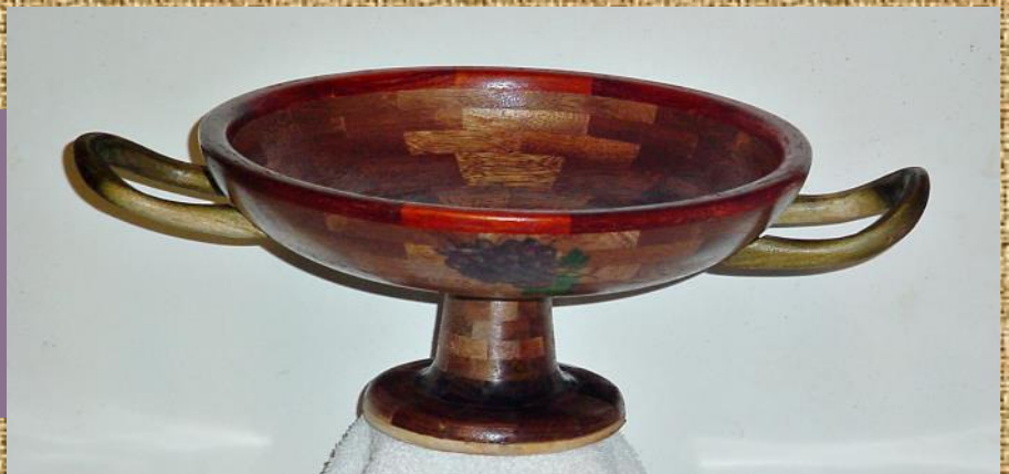
Serving dish made of padauk and sappelle. Handles are poplar and base and stem are of walnut and maple. Barely visible are bunches of grapes applied with ink jet transfer
